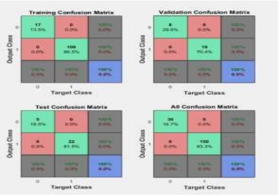
Figure 6: Confusion Matrices of Training, Validation & Testing Phases of the ANN Fault Detector
