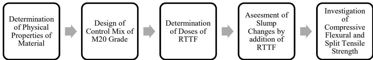
Figure 1: Methodology of Investigation of Properties of RTTF Concrete
