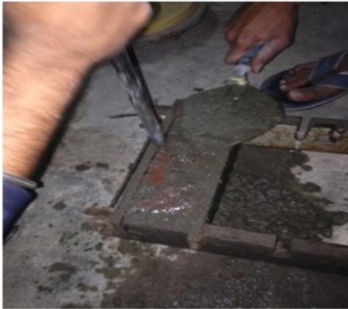
Fig 2: Casting of Specimen
