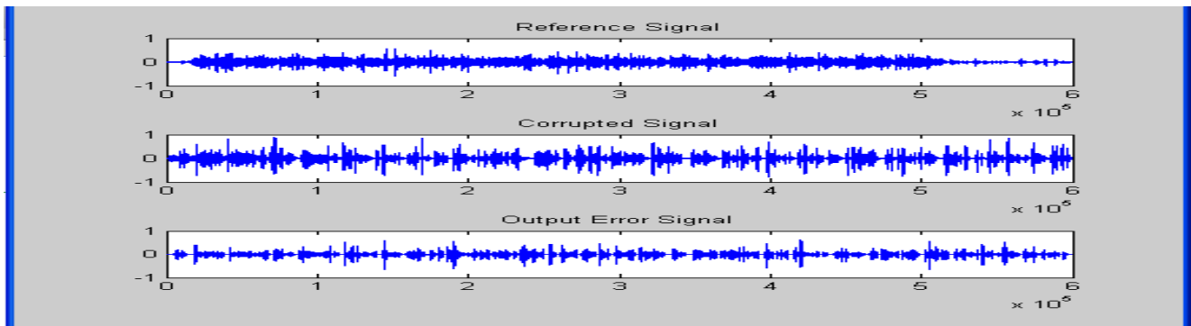
Figure 4: Filtered Speech Signal from Corrupted Vacuum Cleaner Noise
