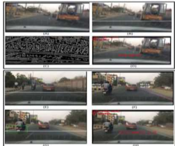
Fig.7 Experimental Result of Road Detection, Vehicle Detection and Alerts in City (A) Original Video Image (B) RoI Generation (C) Edge Detection (D) Warning When Vehicle is too close (E) RoI Generation (F) Road Boundaries detection (G) Detection of Two Wheeler Warning and Alerts
